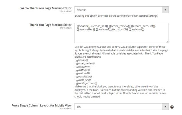
Use **dots** '.' as row separator and **commas** ',' as column separators. Either of these symbols might always be inserted after each variable name to structurize the page. Spaces are not allowed. All available variables associated with Thank You Page blocks are listed below:
